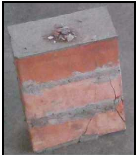
Figura 35. Fisura vertical vista frontal – Semi industrial.
