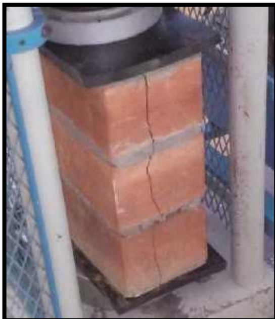
Figura 34. Grieta vertical vista lateral – Semi industrial.
