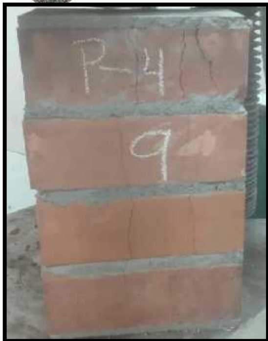
Figura 36. Grieta vertical vista lateral – Semi industrial.
