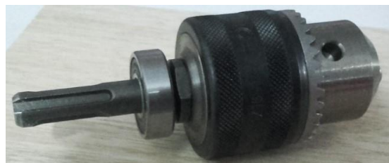
Figura 40: Chuck de taladro 100mm
